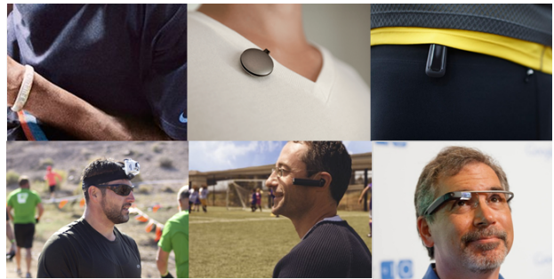
Figure 1: Continuous sensing accessories: Low-datarate (top) accessories based on inertial sensors support self-measurement applications. High-datarate (bottom) ones based on video are restricted to capture/display today.
